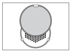
The droplets of fat caught up in the circulating air are deposited on the roasting filter. This helps to keep the oven and the area behind the interior back panel cleaner.
